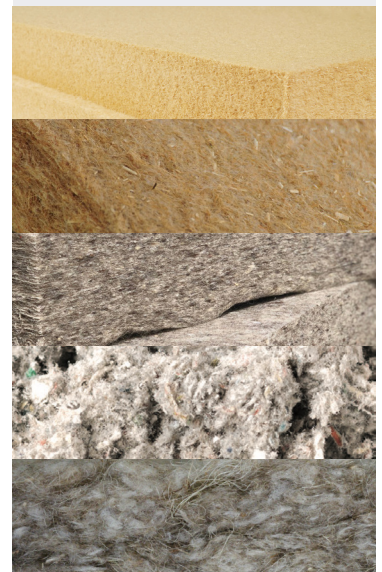
ISOLANTS BIOSOURCÉS Laine de bois: \lambda = 0.036 W/mK, \mu = 2 Laine de chanvre: \lambda = 0.040 W/mK, \mu = 1 Laine de mouton: \lambda = 0.036 W/mK, \mu = 2 Ouate de cellulose: \lambda = 0.038 W/mK, \mu = 1 - 2 Laine de lin: \lambda = 0.038 W/mK, \mu = 1
