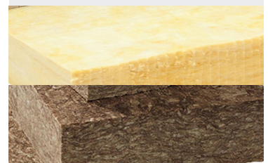
ISOLANTS MINÉRAUX Laine de verre: \lambda = 0.032 W/mK, \mu = 1 Laine de pierre: \lambda = 0.035 W/mK, \mu = 1
